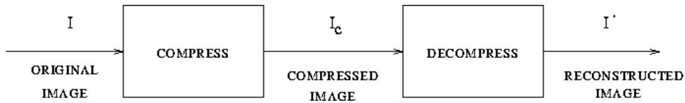
Fig 2 . Image Compression Block Diagram
