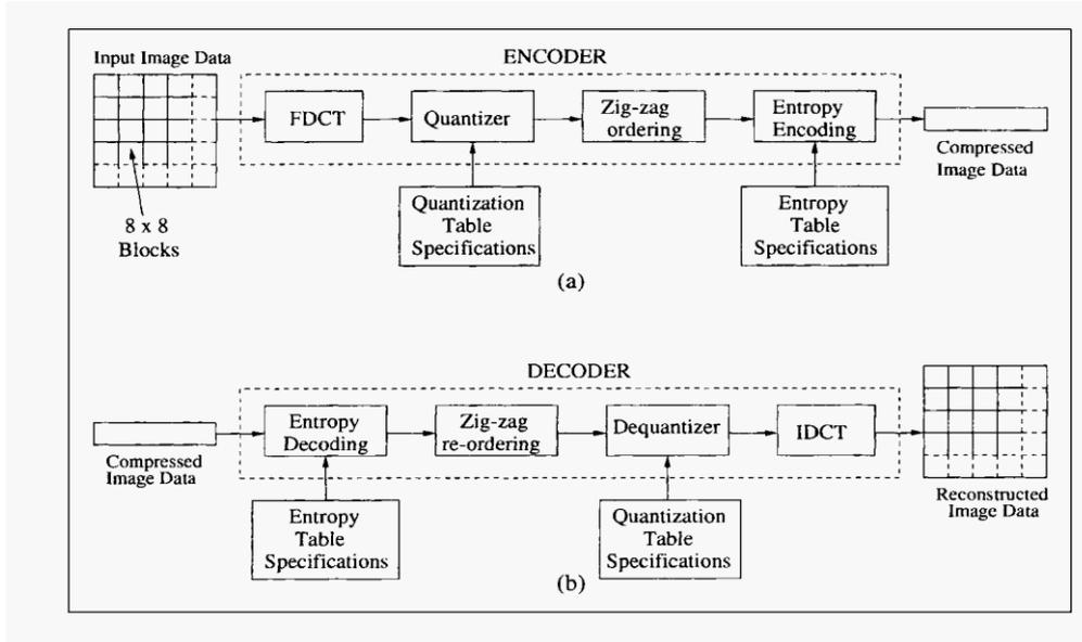
Fig 3. Baseline JPEG: (a)compression, (b) decompression
