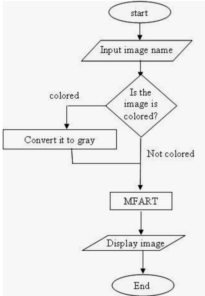
Fig 4.MFART method flowchart
