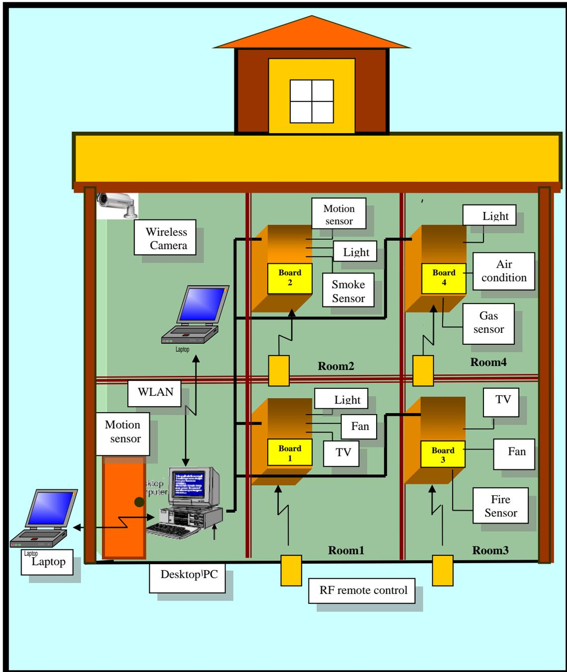
Fig.(1) General Block Diagram of Home Wireless Automation System
