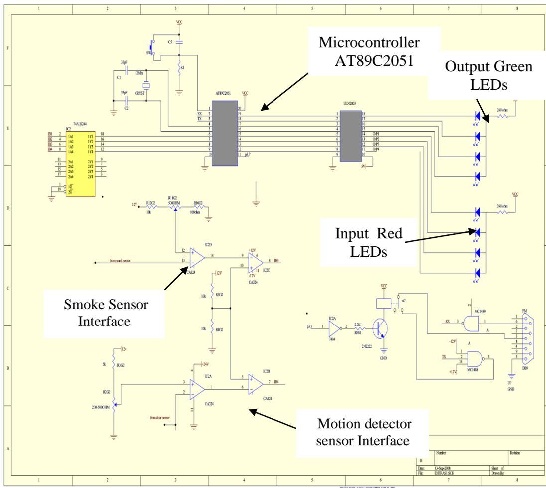
Fig.(3 ) The Schematic Diagram of Board 2
