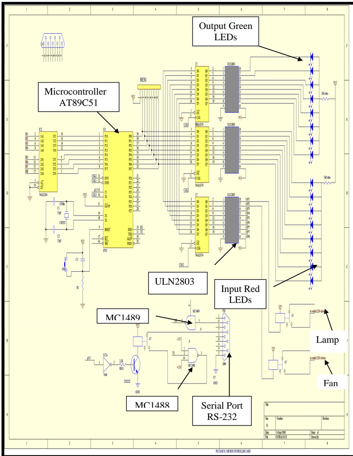
Fig.(2 ) The Schematic Diagram of Board 1
