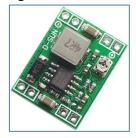
Figure7: 5V-3A Buck Converter
