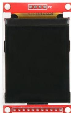
**Figure 8:** Arduino compatible TFT 2.2 colour screen
