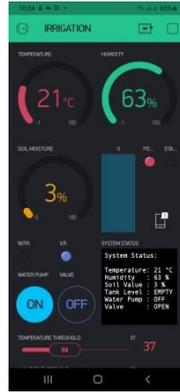
Figure 16: Temperature and Humidity Gauges
