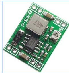
**Figure7:** 5V-3A Buck Converter
