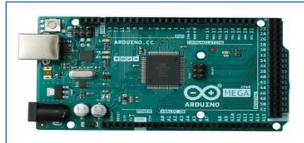
**Fig. 3:** Arduino Mega board
